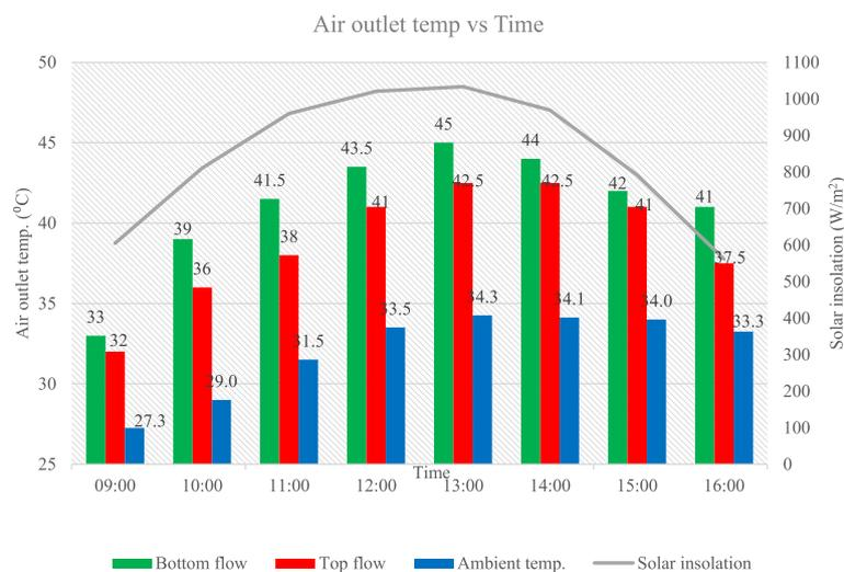
**Fig. 9** Comparison of air outlet temperature for top and bottom flow over the day
