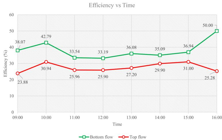
Fig. 10 Efficiency for top and bottom flow configuration
