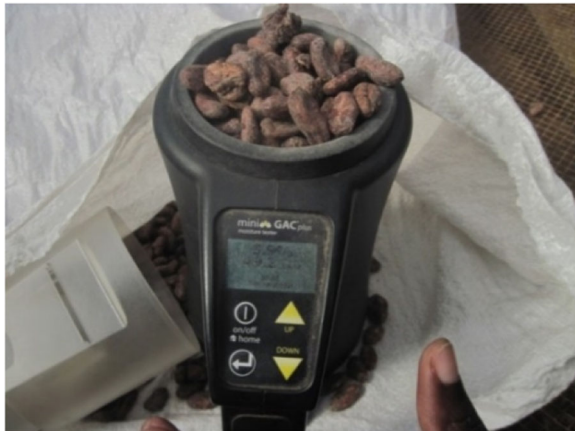
Fig. 4 The determination of the moisture content in the dried cocoa beans using a Dickey John Mini GAC Plus Grain moisture tester
