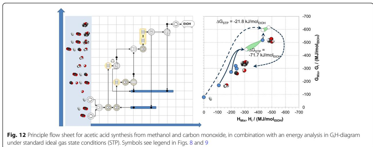
**Fig. 12** Principle flow sheet for acetic acid synthesis from methanol and carbon monoxide, in combination with an energy analysis in G,H-diagram under standard ideal gas state conditions (STP). Symbols see legend in Figs. 8 and 9
