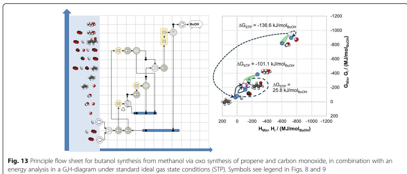
**Fig. 13** Principle flow sheet for butanol synthesis from methanol via oxo synthesis of propene and carbon monoxide, in combination with an energy analysis in a G,H-diagram under standard ideal gas state conditions (STP). Symbols see legend in Figs. 8 and 9
