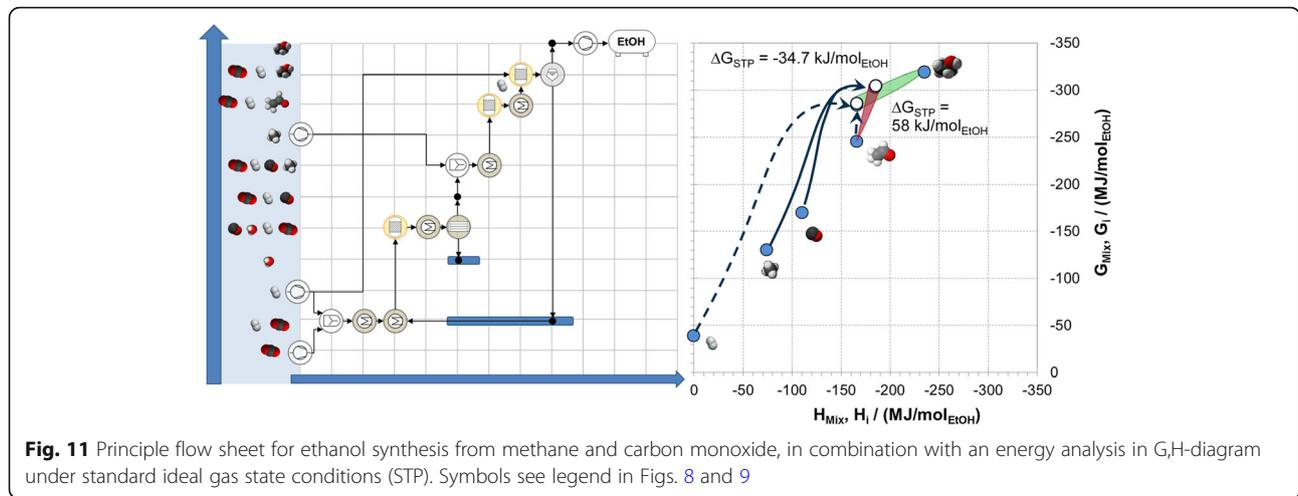
**Fig. 11** Principle flow sheet for ethanol synthesis from methane and carbon monoxide, in combination with an energy analysis in G,H-diagram under standard ideal gas state conditions (STP). Symbols see legend in Figs. 8 and 9
