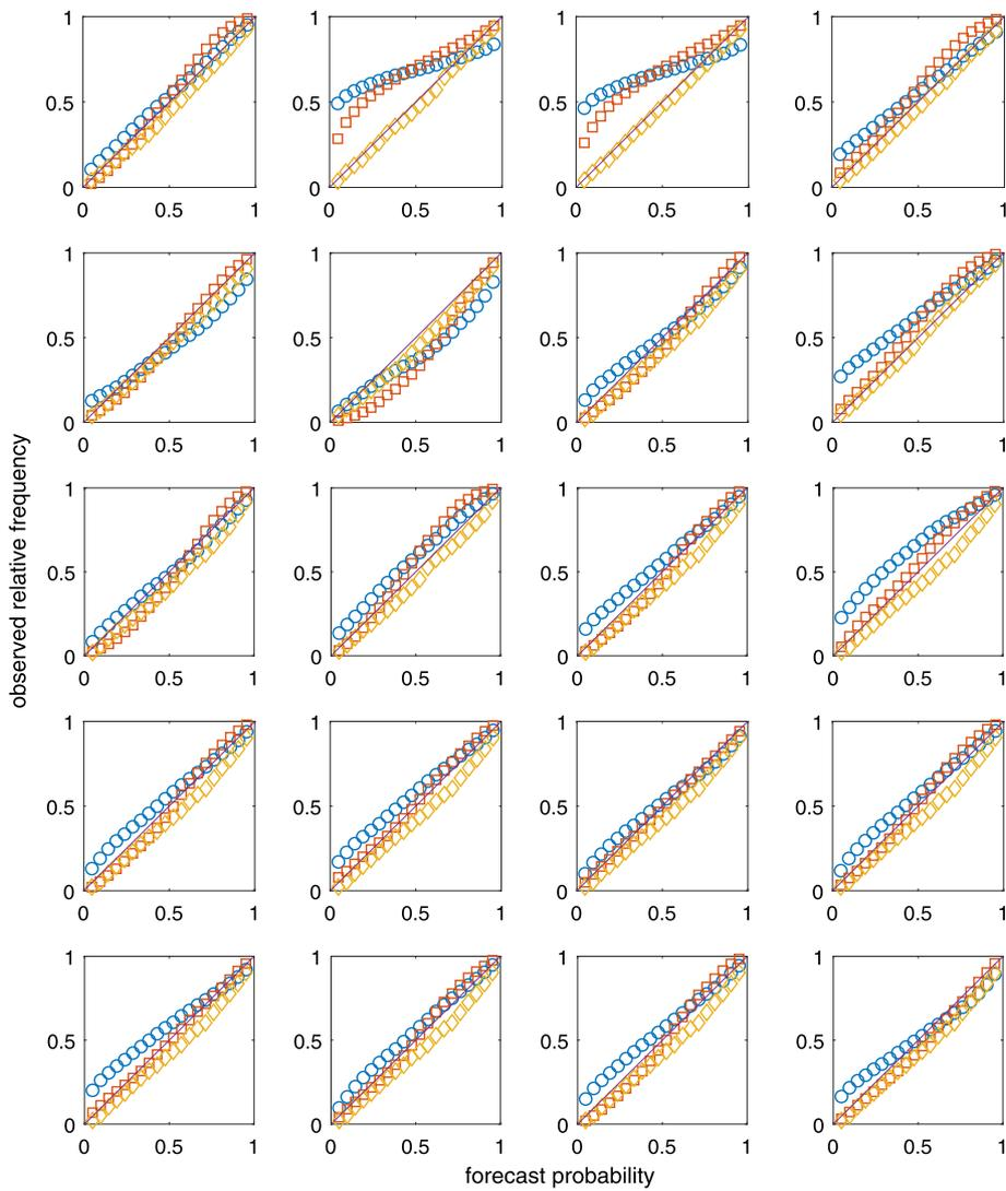
**Fig. 10** Reliability plots of single wind farms in exp. 1 for the three cases: (a) the upscaling without calibration (blue colored circles), (b) the upscaling with calibration (red colored squares), and (c) the hypothetical result of the forecast if data was available for this wind farm (yellow-colored diamonds)
