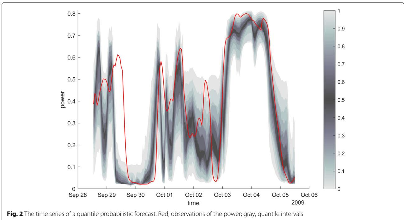
**Fig. 2** The time series of a quantile probabilistic forecast. Red, observations of the power; gray, quantile intervals
