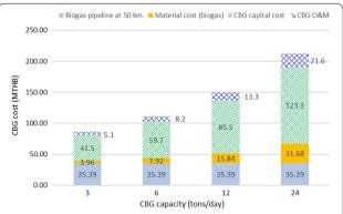
**Fig. 8** The structure of compressed biomethane gas cost (excluded cost of biogas system)
