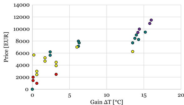
**Fig. 9** A plot of the 28 cases showing  $\Delta T$  and the cost of undertaking the action (in euros). Red dot = 1 action, yellow dot = 2 simultaneous actions, green dot = 3 simultaneous actions, and purple dot = 4 simultaneous actions
