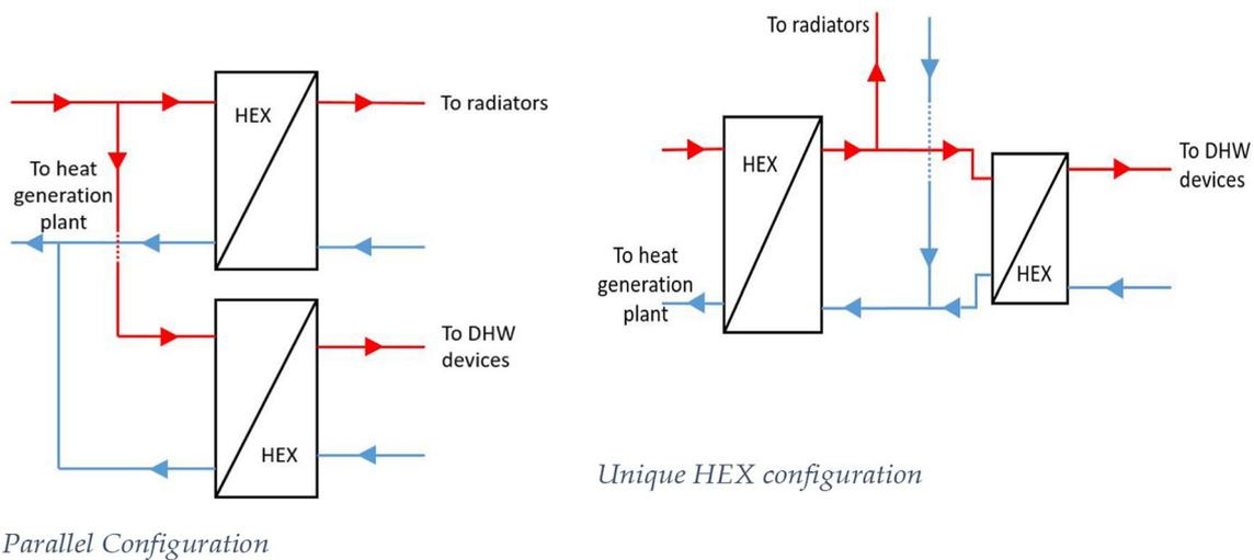
**Fig. 4** Substation architectures
