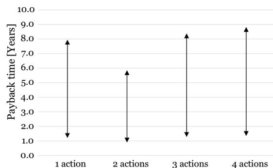
**Fig. 10** Payback times for the best combination of actions for low (20 euro/MWh) and high (130 euro/MWh) gas prices. Actions are 2V (for one action), 2V+LT (for two actions), 2V+LT+parallel (for three actions) and 2V+LT+parallel+instant (for four actions)
