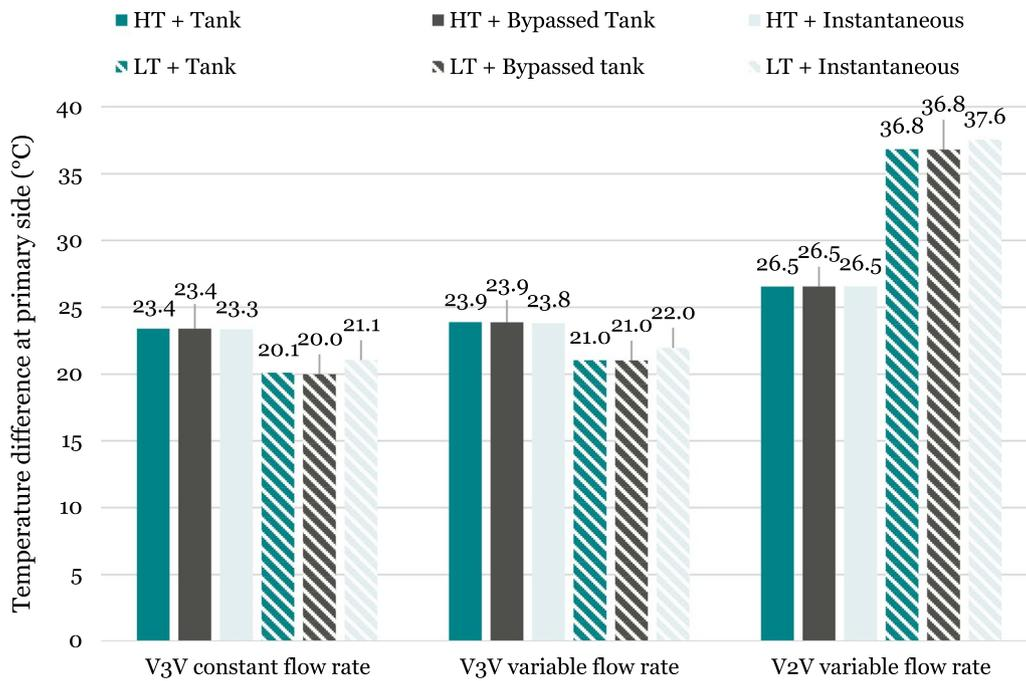
**Fig. 7** Primary  $\Delta T$  comparison for a unique HEX substation
