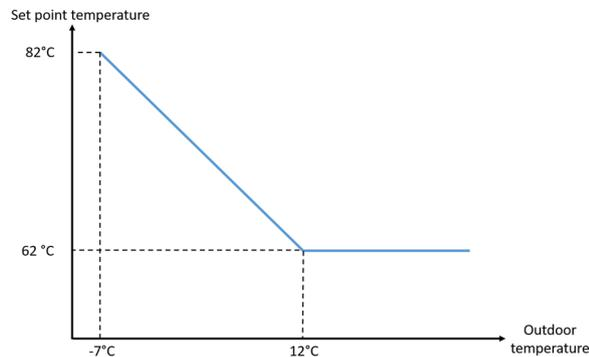
**Fig. 2** Primary supply temperature reset control
