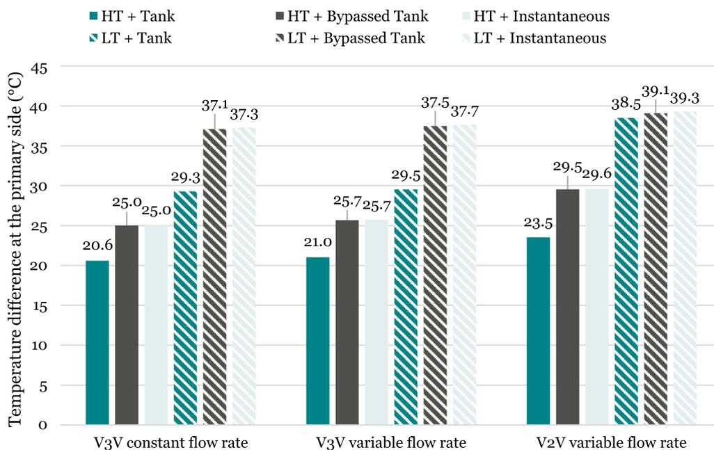
**Fig. 8** Primary  $\Delta T$  comparison for the parallel substation
