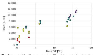
**Fig. 9** A plot of the 28 cases showing  $\Delta$ T and the cost of undertaking the action (in euros). Red dot = 1 action, yellow dot = 2 simultaneous actions, green dot = 3 simultaneous actions, and purple dot = 4 simultaneous actions
