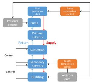
Fig. 1 Structure of the model from the building to the heat generation plant
