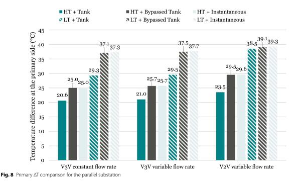
this configuration, the flow at the inlet of the secondary side of the HEX comes directly and exclusively from the hot water tank (T = 60 °C), in contrast to the two other configurations. In these cases, the secondary flow at the HEX inlet can come not only from the hot water tank but also from the cold-water network and the recirculation line, thereby allowing for a reduction in return temperature.
