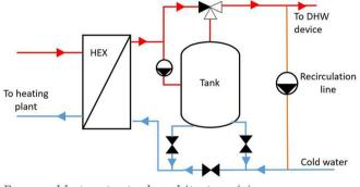
*Bypassed hot water tank architecture (c)* **Fig. 6** DHW architectures
