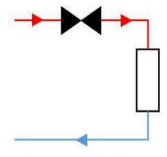
*Two-way valve control (V2V)* Fig. 5 Radiator control systems
