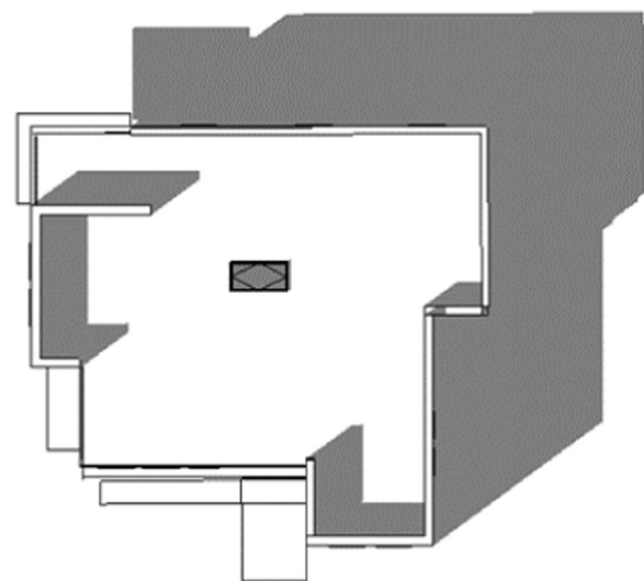
Fig. 6 Roof area for PV system (design 1,3B)
