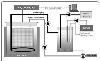
Figure 3 A schematic of the lab-scale biogas reactor with biomass recirculation and pH control.
