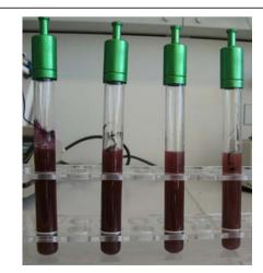
Figure 6 TTC test with the used microbes in the presence of the industrial desizing liquor.
