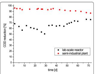
**Figure 8 Time-dependent COD reduction of industrial desizing liquors.** Time-dependent COD reduction of industrial desizing liquors from cotton pretreatment in a lab-scale and a semi-industrial biogas reactor.
