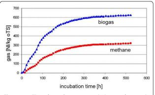
**Figure 7 Time-dependent gas emission under static fermentation conditions.** The gas volumes were corrected by the gas generation of the seeding sludge.
