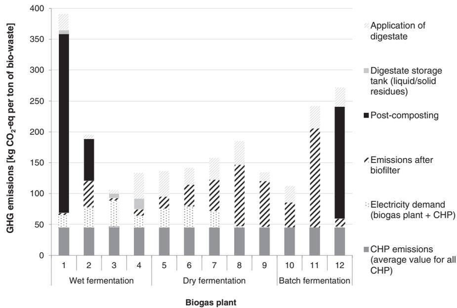
**Figure 2** GHG emissions of bio-waste digestion plants differed to kind of plant components. The GHG emissions are presented in kg CO<sub>2</sub>-eq per ton of bio-waste differed to the kind of fermentation process (wet, dry, or batch fermentation) and the main emission sources within the process chain.
