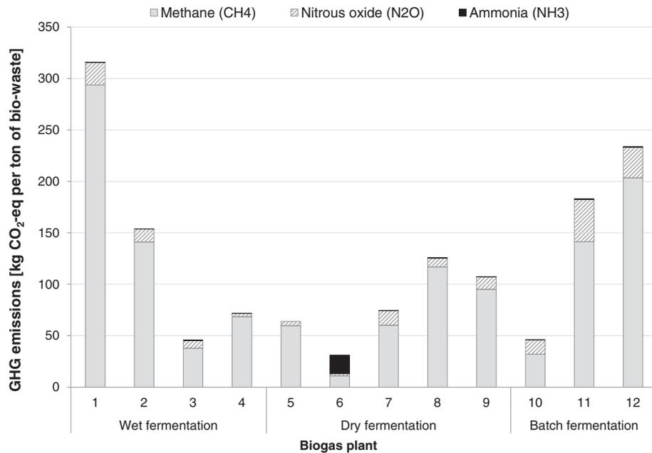
**Figure 1** GHG emissions of the investigated biogas facilities (bio-waste) differed to the kind of GHG emission. The measured emissions of investigated AD plants are presented in kg CO<sub>2</sub>-eq per ton of bio-waste differed to the kind of GHG emission and kind of fermentation process. Methane and nitrous oxide emissions = direct GHG emissions, ammonia = indirect GHG emissions.
