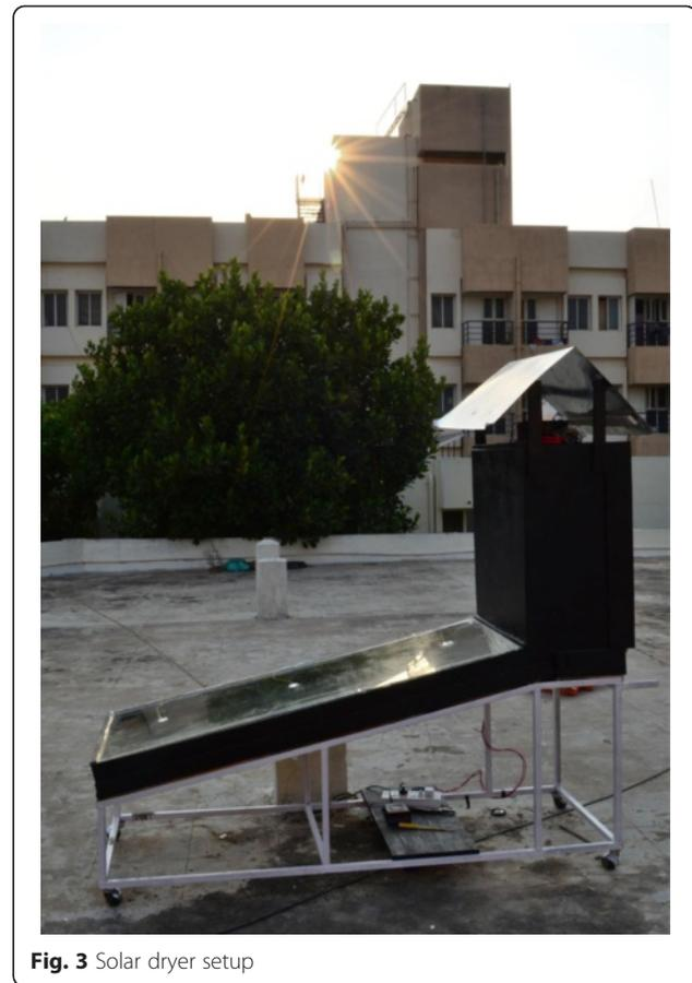
**Fig. 3** Solar dryer setup
