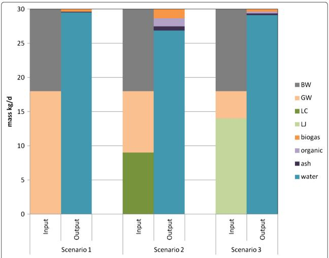
Fig. 5 Mass balances for the three scenarios with different feed mixtures and corresponding outputs for the Jenfelder Au situation. Output: digestate (composed from water, ash and organic) and biogas
