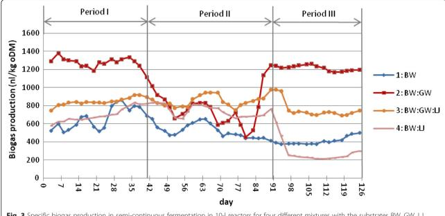
Fig. 3 Specific biogas production in semi-continuous fermentation in 10-l reactors for four different mixtures with the substrates BW, GW, ⊔ during three different feeding periods
