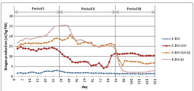
Fig. 2 Absolute biogas production in semi-continuous fermentation in 10-l reactors for four different mixtures with the substrates BW, GW and LJ during three different feeding periods
