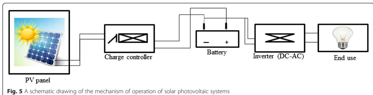
**Fig. 5** A schematic drawing of the mechanism of operation of solar photovoltaic systems
