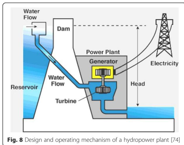
**Fig. 8** Design and operating mechanism of a hydropower plant [74]
