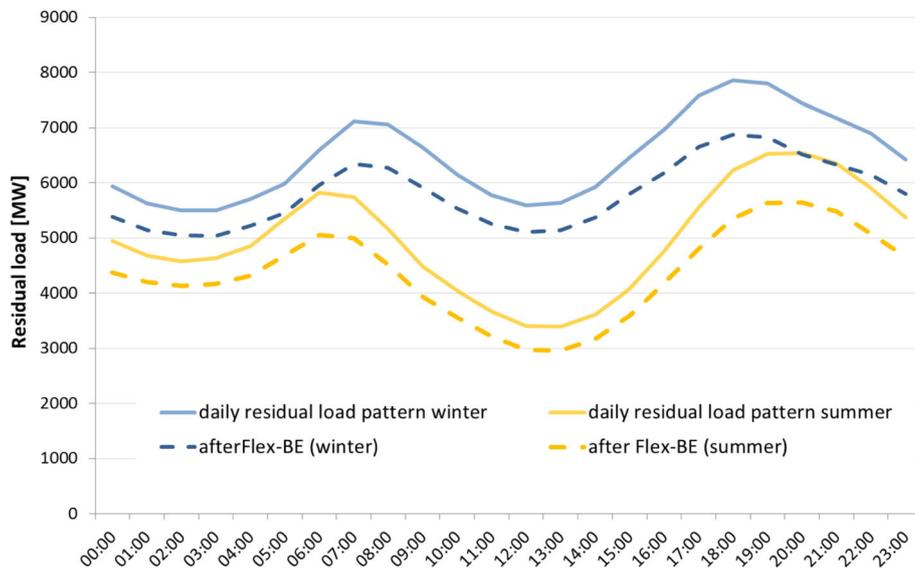
**Fig. 3** Daily residual load before and after flexible power generation from biomass, differentiated for winter and summer time. (Note the reduced amplitude in average daily RL after flexible bioenergy power generation and the typical reduction of RL at noon in summer time which is partially caused by high solar PV feed-in)
