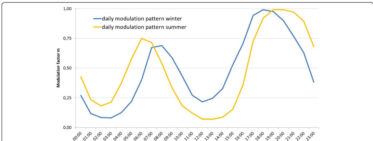
**Fig. 2** Average modulation of cluster 2 (biogas plants and liquid CHP plants) over the course of the 24 h of the day, differentiated for winter and summer time. (Note the typical reduction of modulation at noon, especially pronounced in the graph depicting summer time modulation, caused by high solar PV feed-in; Additionally the earlier and later modulation peak during summer time compared to winter time)
