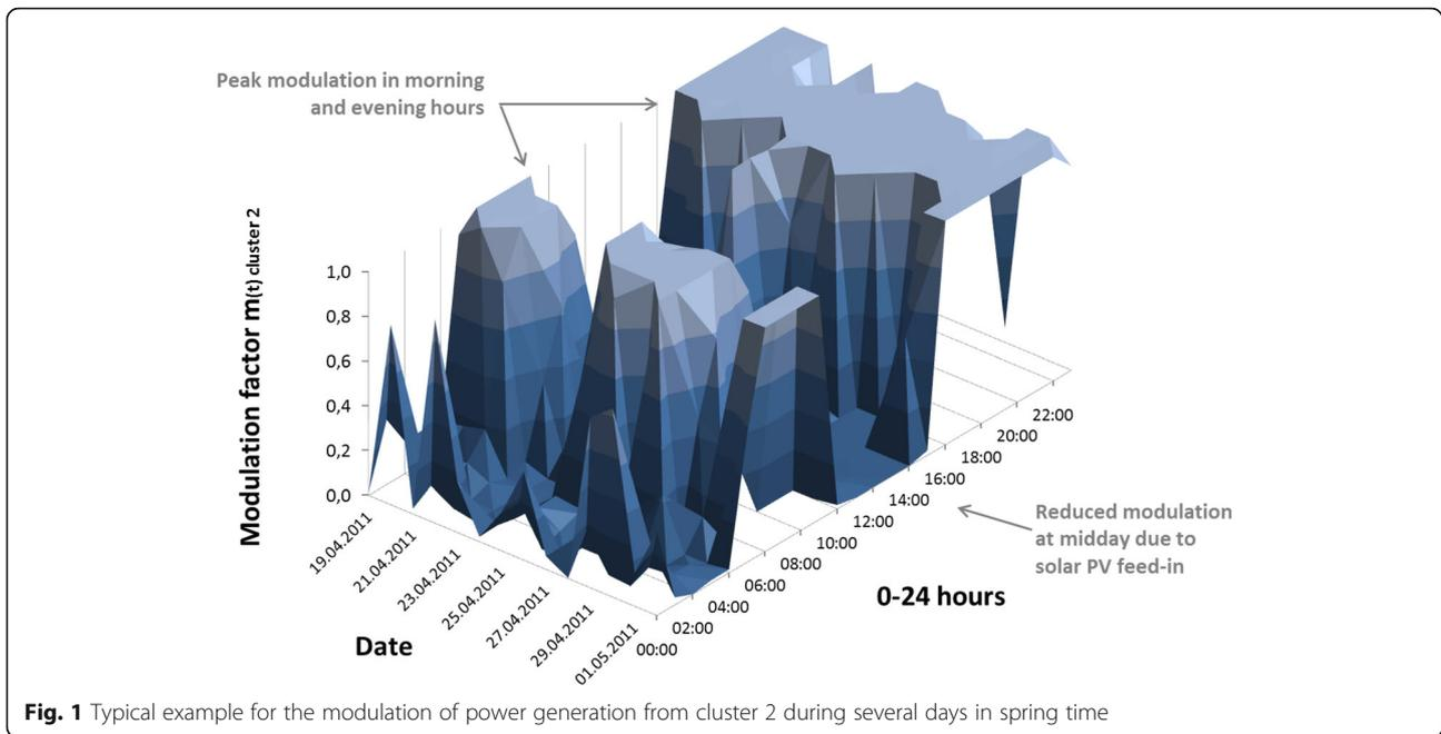
**Fig. 1** Typical example for the modulation of power generation from cluster 2 during several days in spring time
