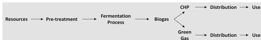
**Fig. 1** Schematic representation of typical biogas production chains
