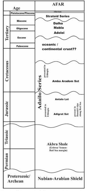
**Fig. 2** Simplified stratigraphy of Afar. In Djibouti, the Eocene and post-Eocene members directly lie over the Oceanic/Continental basic crust (adapted after [16])
